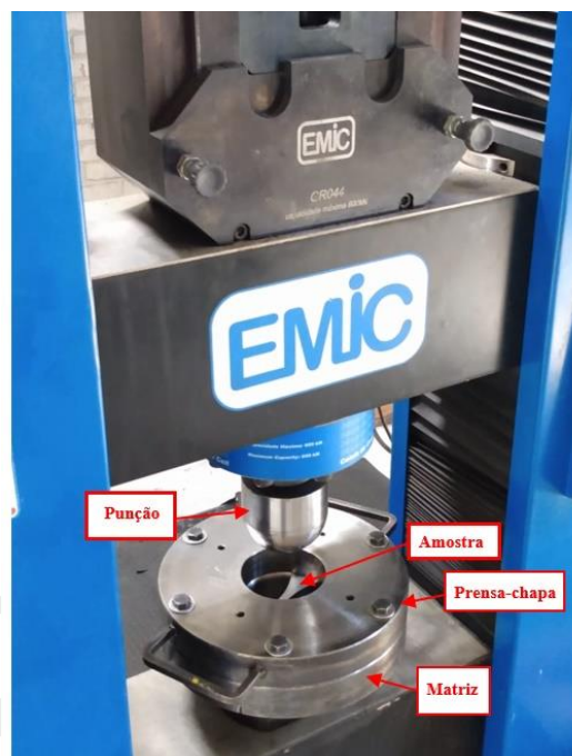
Figure 11 – Representation of the modified Nakazima test performed on the EMIC machine.
